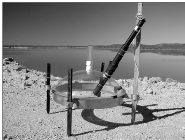
Figure 4 —Assembled dome and probe/logger ready for use.
